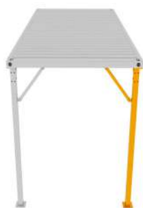
1 Right column 2x 2.2m Made of 100x100x5mm tubes
