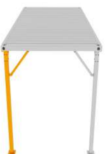
4 Left column 2x 2.4m Made of 100x100x5mm tubes
