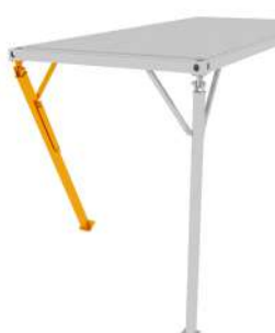
8 Foldable Left 2x 3.0m Made of 100x100x5mm tubes
